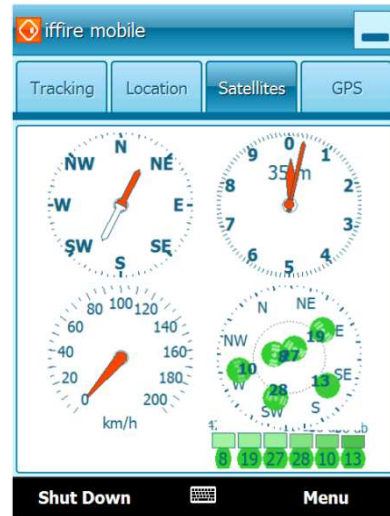
9 - Current satellites info Info about satellites available, direction, speed and altitude.
